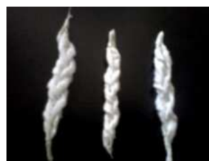
Fig. 3. Single braided-twisted fibers
