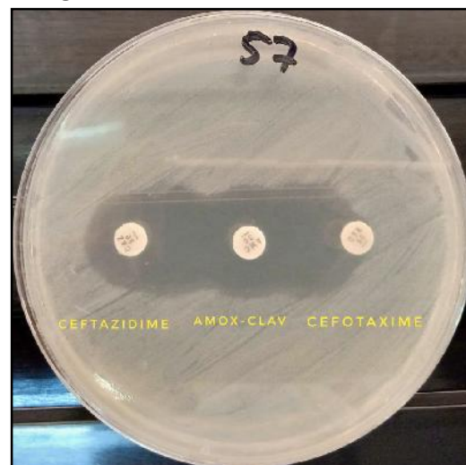
Fig 1. Double Disc Synergy Test (DDST) for ESBL confirmation
