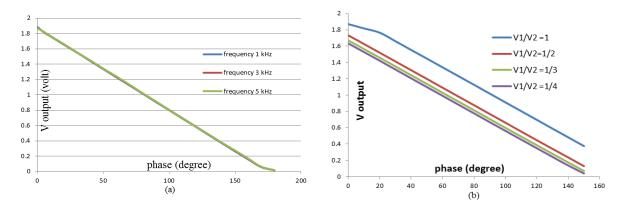
**Figure 11.** (a) The relation of the linearity of phase differences and voltages from signals detector with the same amplitude. (b) The linearity graph of phase detector's voltages to the phase differences for two different signal amplitudes.
