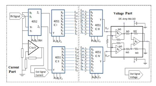
Figure 6. The electric mechanism for selecting a current injector electrode and measuring voltage.
