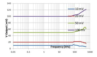
**Figure 10.** The stability of root mean square (RMS) to direct current (DC) circuit of output voltage to DC against frequencies.
