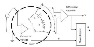
**Figure 3.** The scheme in the measurement of impedance components separately through a measurement of voltage and phase difference.
