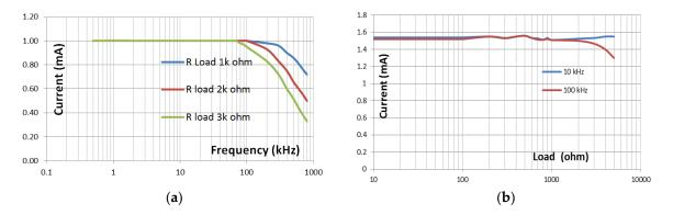
frequencies up to 150 kHz. At the frequencies of 150–200 kHz, there is a 1% decrease in amplitude from the stable state. The 2 k $\Omega$  load on VCCS is stable until 100 kHz while for the 3 k $\Omega$  load reaches 80 kHz.
