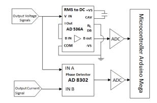
Figure 7. Measurement scheme of voltage and phase difference.
