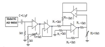
Figure 5. A signal generator and constant current.
