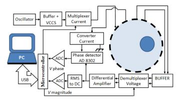
Figure 4. Block diagram of Electric Impedance Tomography System for real and imaginary functional images.
