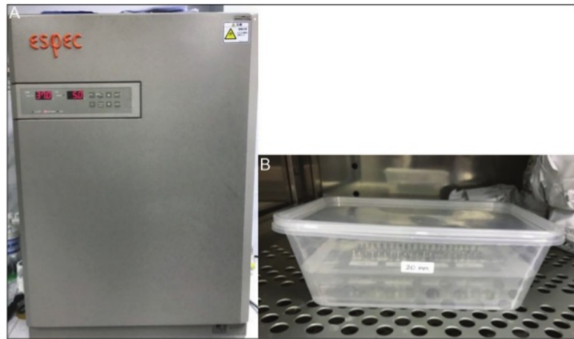
Figure 2: (A) Precision incubator with 37°C temperature (Especc, North America). (B) Elastomeric chains were submerged in water baths housed in an incubator
