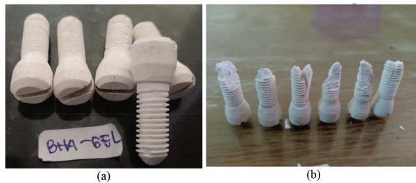
Fig. 4. The printed bio-screw (a) before and (b) after the compressive strength test
