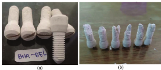
Fig. 4. The printed bio-screw (a) before and (b) after the compressive strength test
