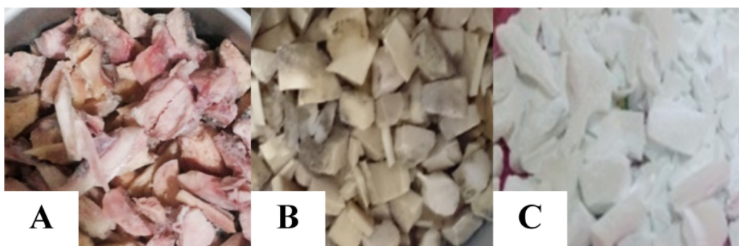
Fig 1. The representative physical appearances of raw bone materials before boiling process (A) and after pressurized boiling process (B), and end hydroxyapatite product after calcification (C).
