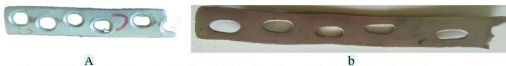
Fig. 1. (a) As-cast implant plate 316L and (b) implant plate 316L after 50% reduction by cold rolling
