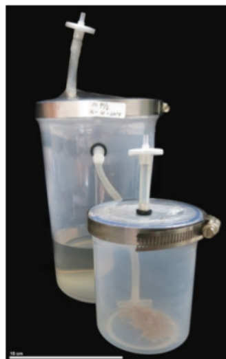
Fig. 1: Temporary immersion bioreactor modified from 23 BIT®
