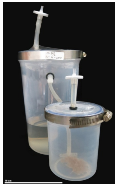
Fig. 1: Temporary immersion bioreactor modified from 23 BIT ®
