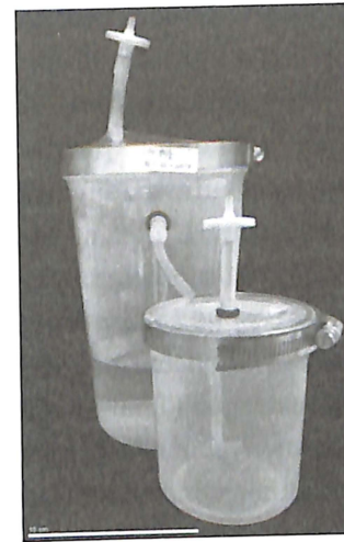
Gambar 3. Bioreaktor Perendaman Sementara ( Temporary Immersion Bioreactor ).
