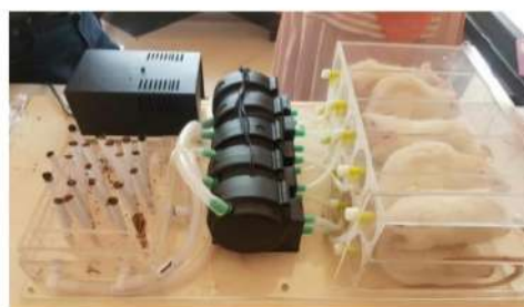
Figure 1. The process of handling experimental animals exposed to cigarette smoke with a device of full-body exposure.
