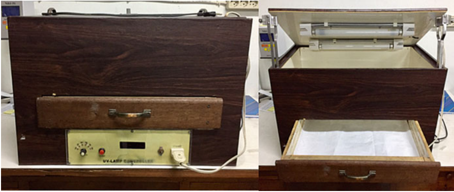
Fig. 1 Wooden box with TL20W/12RS UV lamp installed at the top of the box. The distance of the lamp was 20 cm from the back of the animals
