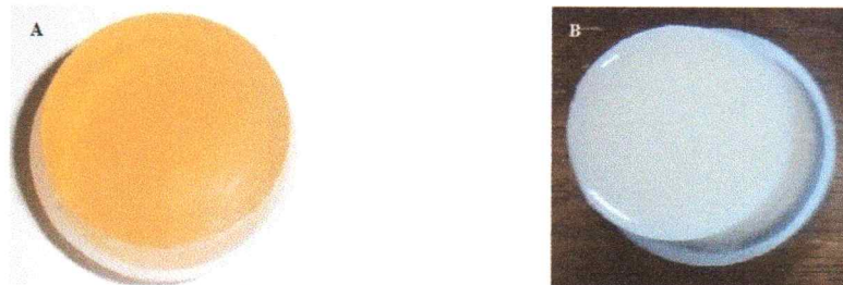
Figure 1. Phantom Gelatin-glycerin (a) without the addition of TiO_2 (b) the addition of 0.01 grams TiO_2
