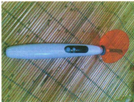
Gambar 4.1 : Light curing unit komposit merk woodpecker, sinar LED .
