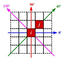
Fig. 2 The four different orientations for generation of GLCM
