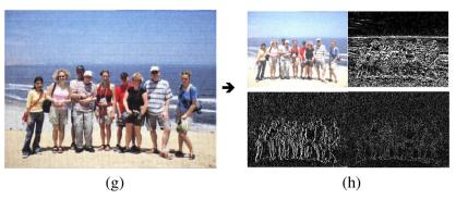
Fig. 4 Different sub-bands after DWT. (a) original printed image. (c), (e), (g) are the scanned images from different color laser printers. (b), (d), (f), (h) are the wavelet sub-bands of (a), (c), (e), (g) respectively after 1 level DWT decomposition
