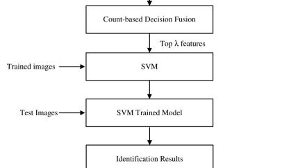
Fig. 5 Procedure of identifying source laser printers
