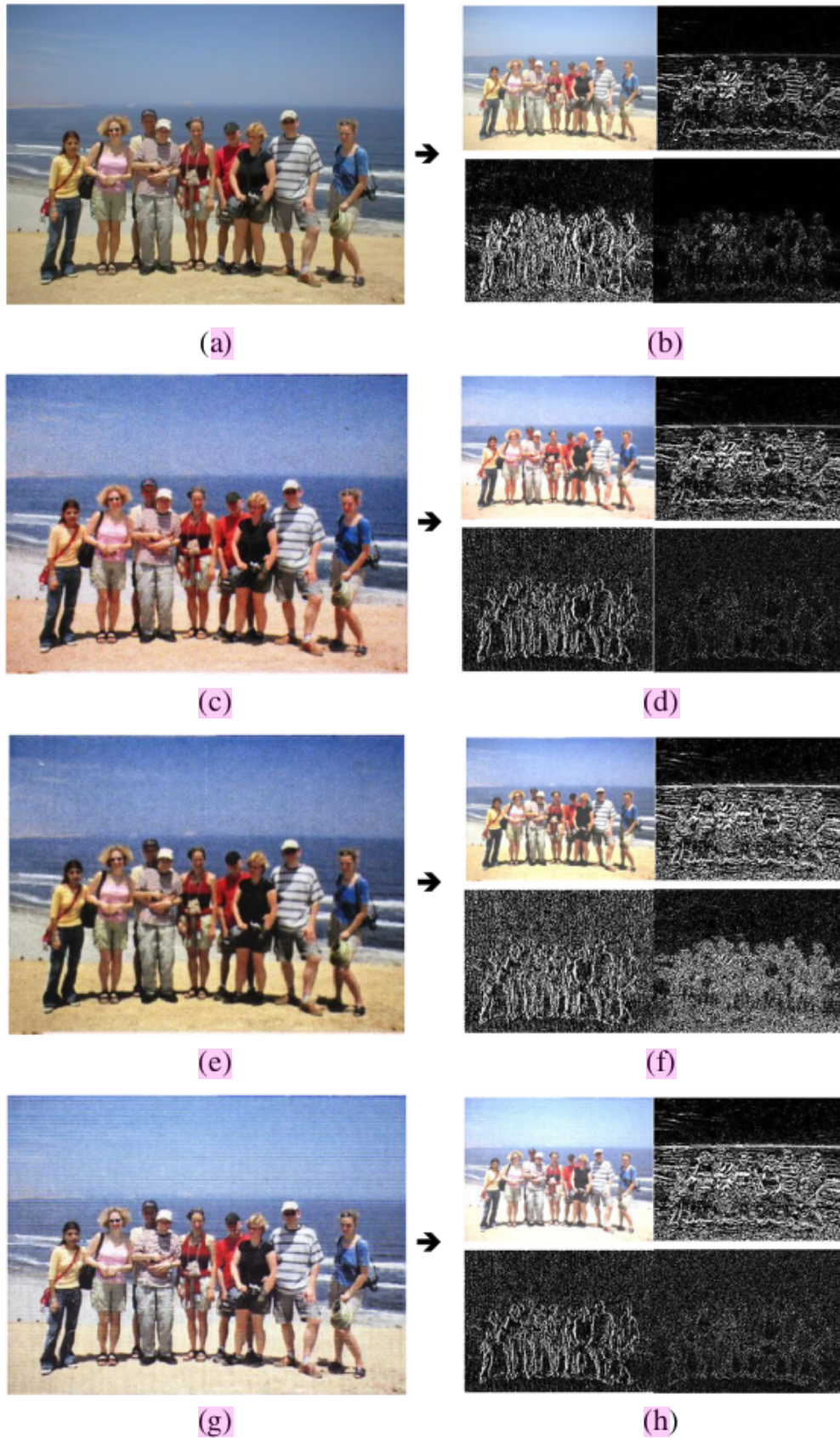
Fig. 4 Different sub-bands after DWT. (a) original printed image. (c), (e), (g) are the scanned images from different color laser printers. (b), (d), (f), (h) are the wavelet sub-bands of (a), (c), (e), (g) respectively after 1 level DWT decomposition
