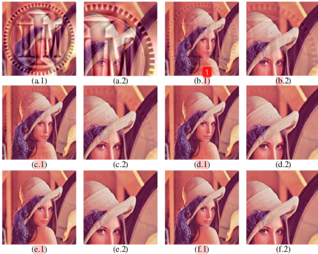
Fig. 7 The visual quality comparison for different \delta value of watermarked Lena images. (a.1), (b.1), (c.1), (d.1), (e.1) and (f.1) are watermarked Lena images with \delta=0, 0.5, 0.7, 1.0, 1.2, 1.5 respectively. (a.2), (b.2), (c.2), (d.2), (e.2), and (f.2) are close-up images of (a.1), (b.1), (c.1), (d.1), (e.1), and (f.1) respectively. The PSNRs of (a.1), (b.1), (c.1), (d.1), (e.1), and (f.1) are 17.43 dB, 28.86 dB, 32.52 dB, 36.21 dB, 37.67 dB and 39.11 dB respectively
