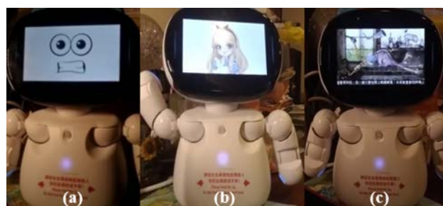
Figure 4. Developments of robot-based storytelling systems: (a) designing facial expressions, (b) setting characters of a story, and (c) constructing story context.
