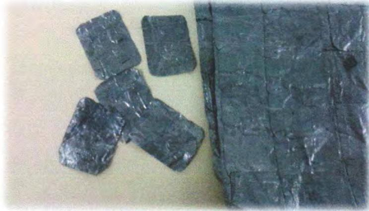
Gambar 5.1.1 Limbah lead aluminium film dental
