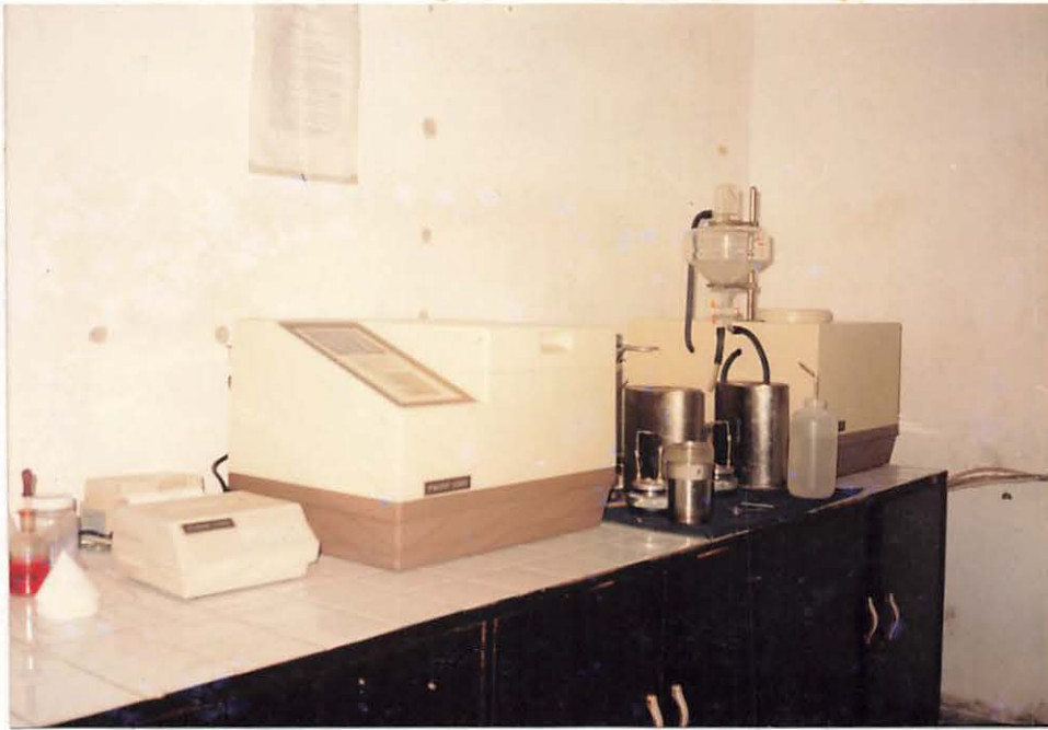
Gambar 3. oksigen bom kalori meter berdasarkan ASTM - D 2015 - 91
