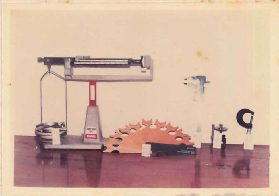
1. Timbangan Ohaus. 2. Ovocolor fan. 3. Jangka sorong. 4. Spherometer. 5. Caliper micrometer.
