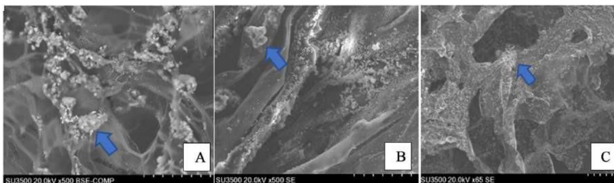
Figure 4. HAp-Col-EGCG scaffold with 1% (A), 2% (B), and 4% (C) showed interconnected pores and agglomerated HAp dispersed in a the scaffold
