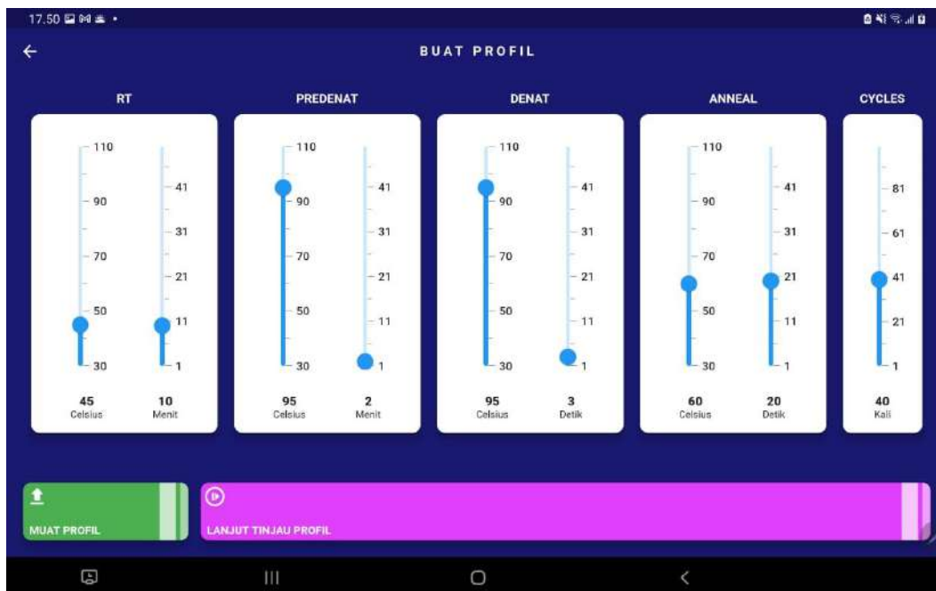
Gambar 40. Tampilan setting protokol temperatur GUI rRTPCR
