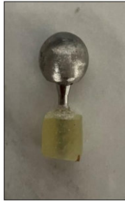
Figure 2 Ti-6Al-4V implant with implant holder made of ARALDITE® Standard Setting Epoxy Glue and specimen head made of VERABOND® Nickel Chromium
