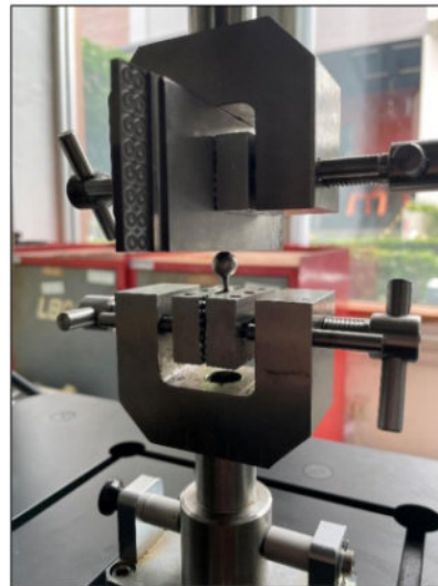
2 Figure 4 The compressive test of T1-6Al-4V using the universal testing machine Hung Ta Type HT-9501
