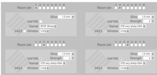
Figure 1 : Parameter Setting in FBP B70F Sharp and SAFIRE I70f (level 2,3,4). The data were, then, collected and reconstructed by using kernel filter B70f sharp lung window and SAFIRE soft tissue standard I70f sharp level 2,3 and 4. Various studies using FBP B70F Sharp as a standard filter in Chest HRCT reconstruction because it can increase spatial resolution which is an important aspect in Chest HRCT.
