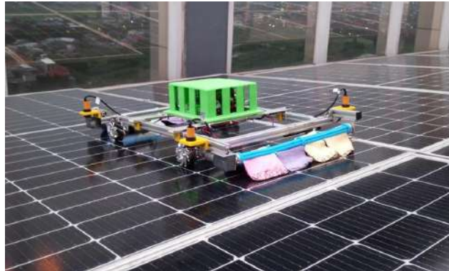
Gambar 3.3. Robot ARVOS ( Photovoltaic Array Sweeper )
