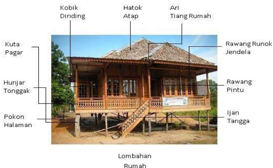
Figure 3.2. Parts of a Stilt House
