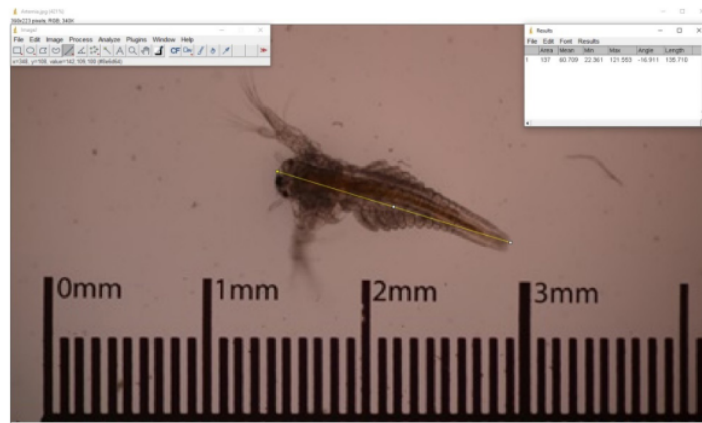
FIGURE 2. A scaled photograph of Artemia taken using a DSLR camera under a dissecting microscope as a raw material for measurement of total length using ImageJ software
