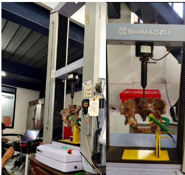
Figure 2. Biomechanical Testing of Cadaveric Pelvic Bone Using Autograft. A particular holder device was made to fix the pelvic during the experiment.
