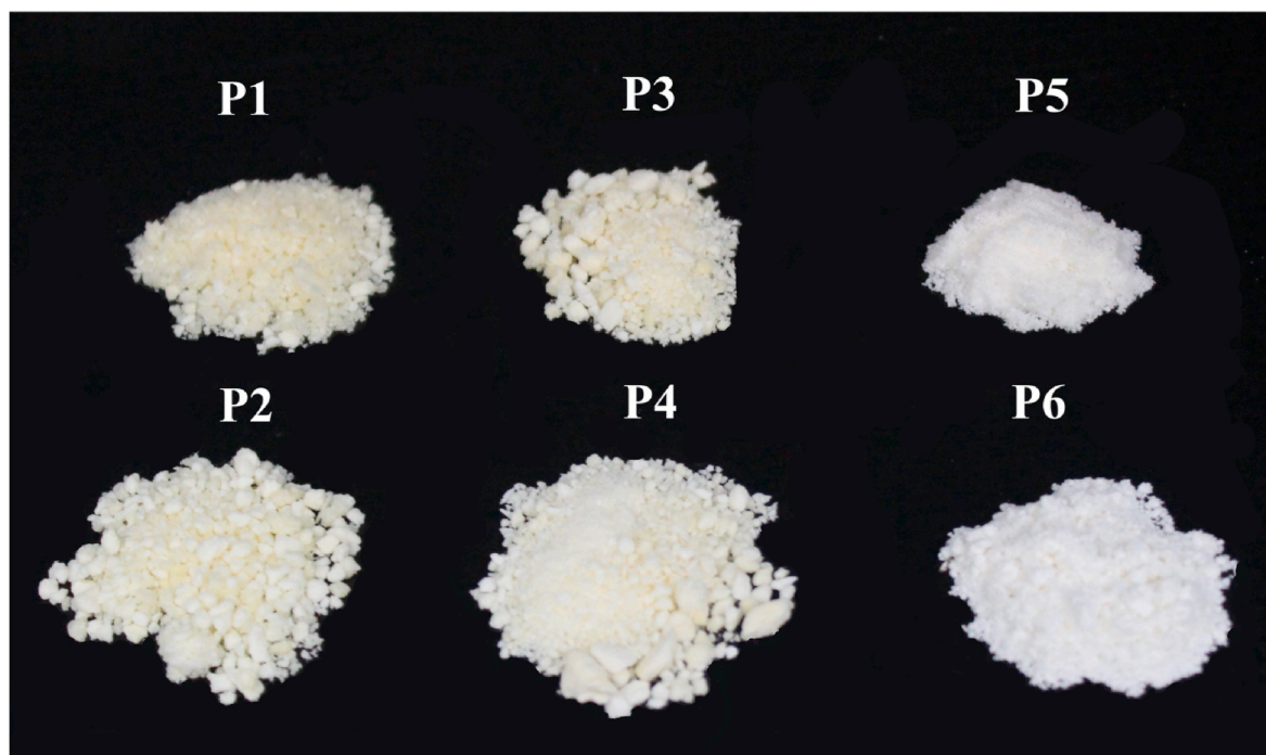
Fig. 3. Microencapsulated tuna fish oil powder from (P1) Maltodextrin: Whey Protein (5.0:1.0) as control; (P2) Maltodextrin: Whey Protein (6.5:1.0) as control; (P3) Arrowroot starch: Whey Protein (5.0:1.0); (P4) Arrowroot starch: Whey Protein (6.5:1.0); (P5) Maltodextrin: Arrowroot Starch: Whey Protein (3.344:1.668:1.0); and (P6) Maltodextrin: Arrowroot Starch: Whey Protein (3.25:3.25: 1.0).
