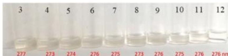
Fig. 1. Photos of NBP under various pH ranges (from pH 3 to pH 12). The UV absorbance maximum of each sample is showed in the lower series
