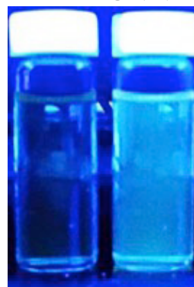
Fig. 2. (a) Emission Spectra of FC; (b) photograph images of water (left) and FC 300 (right) under 254 nm UV light.
