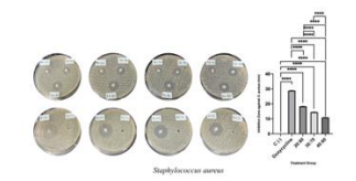
Fig. 2 Antibacterial inhibition zone of PMMA-HA scaffold with ratios 20:80, 30:70, and 40:60 against Staphylococcus aureus
