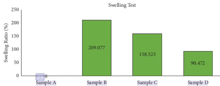
FIGURE 2: The swelling test results of hyaluronic acid (HA): chitosan hydrogel with varying composition HA: chitosan sample A (30 : 0 mg/ml), sample B (30 : 10 mg/ml), sample C (30 : 20 mg/ml), sample D (30 : 30 mg/ml).
