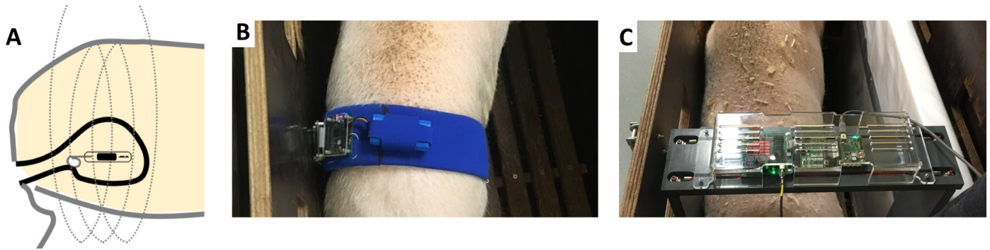
Fig 2. Principle of Bladder Pill for pressure measurement in animals. (A) Diagram of working mechanism of Bladder Pill in vivo, wireless induction as represented by coils (dotted lines) contained within a corresponding external device. (B) Waistband-form external device tested in vivo. (C) Rectangular frame.
