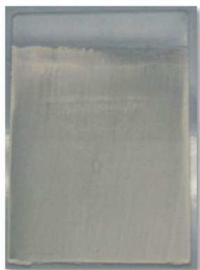
Fig. 8. The coating results of TiO 2 on the glass plate with doctor blade method.
