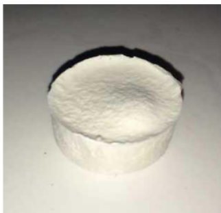
Figure 1. Nano-hydroxyapatite-chitosan carboxy-methyl Cellulose (CMC) Composite Scaffold.
