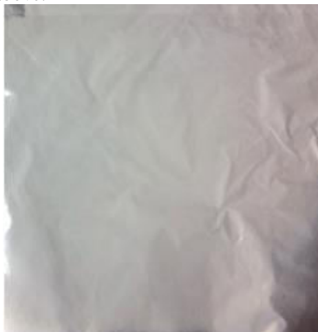
Figure 2. Electrospun PVA- Aloe vera -Based Nanofiber Membrane on the Aluminum Foil
