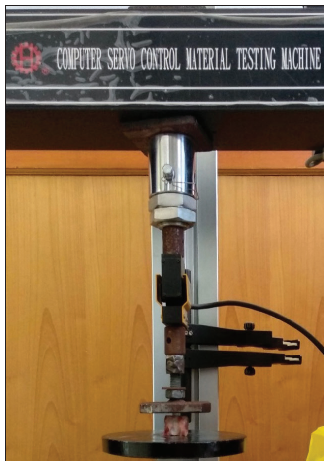
Figure 1: Mechanical testing machine that used in the compression test of the lumbar vertebrae body.
