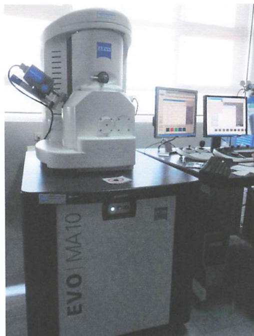
Gambar 2 Alat Scanning Electrone Microscope (SEM) EVO MA10
