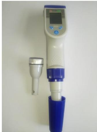
**Gambar 2.1** Alat Digital Water Tester XPT-8
