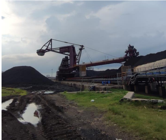
Gambar 4.8 Stacker Reclaimer PT. POMI (Data primer, 2022)
