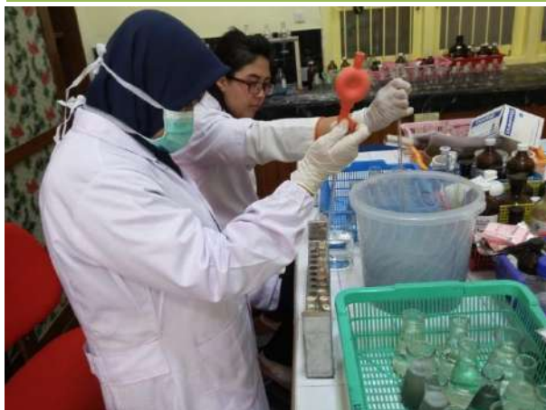
Gambar 6.11 Persiapan Sampel Air Limbah Uji COD
