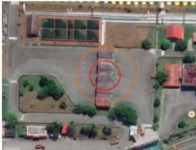
Gambar 4.3 Denah Fatality Zone dan Injury Zone di Filling Shed
