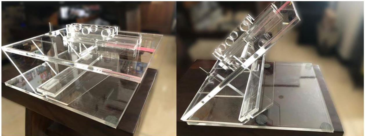
Figure 7: Tilt-adjustable acrylic intubation base
