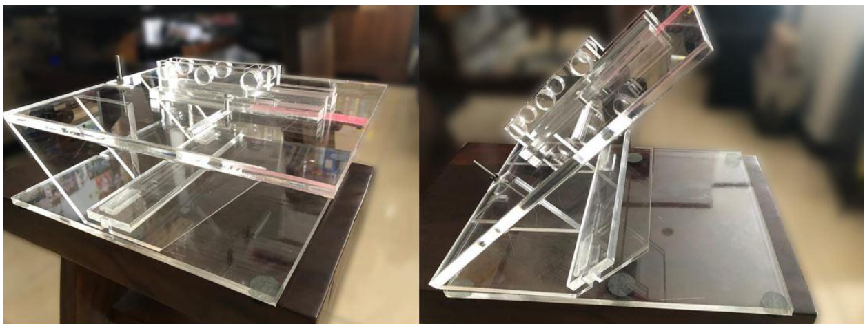
Figure 3: Tilt-adjustable acrylic intubation base
