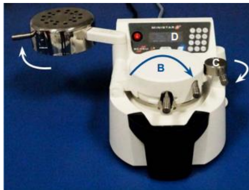
Gambar 2.7 penguncian presser chamber ( https://www.greatlakesdentaltech.com/ )
