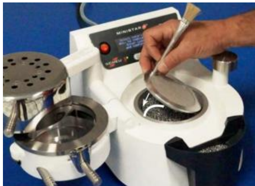
Gambar 2.6 Persiapan pellet cup / pemasangan platform ( https://www.greatlakesdentaltech.com/ )
