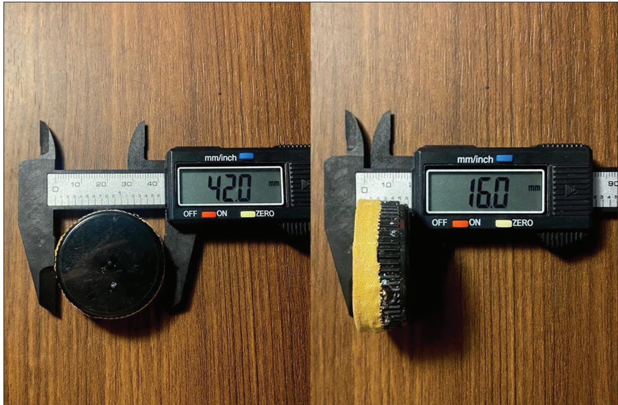
Fig. 1. Occluding device design with measurement.
