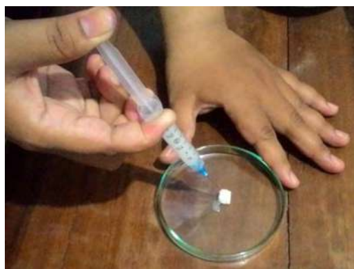
Gambar 3.4 Proses pengujian Setting time
