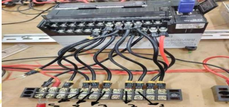
Gambar 4.7 Hasil *wiring input*
